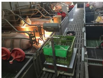
Another example of a piglet care trolley with built-in scale for litter weighing.
